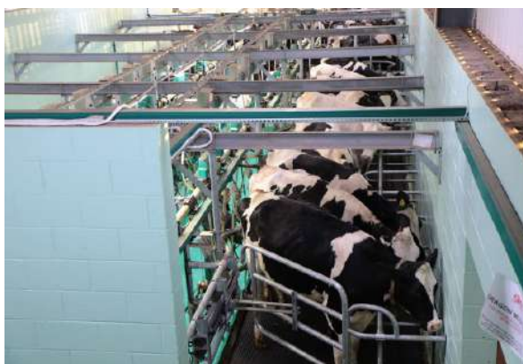
Fig. 3.10: Cattle being milked by a milking machine
